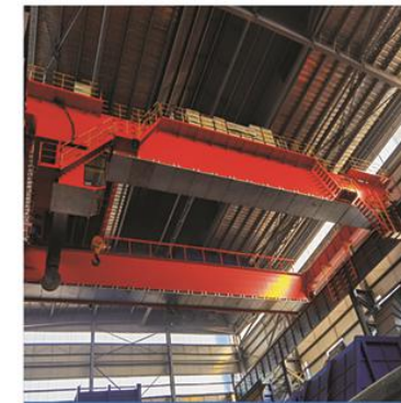
200吨行车 200 tons Travelling crane
